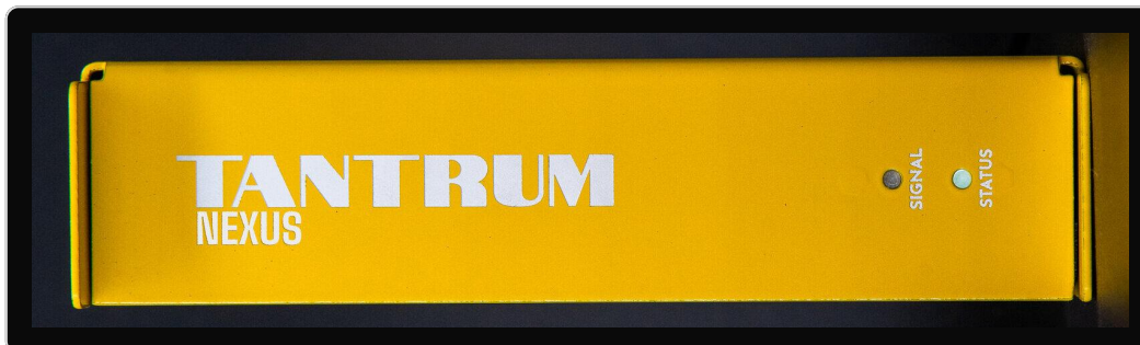
NEXUS front panel: SIGNAL and STATUS LEDs on the right
