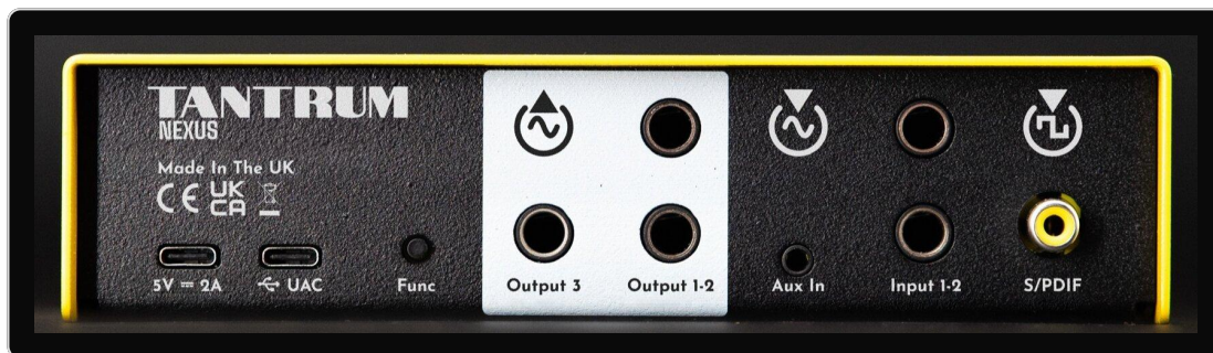
NEXUS rear panel, left to right: 5V 2A, UAC, Func, Output 3, Output 1-2, Aux In, Input 1-2, S/PDIF
